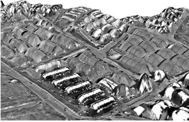
Figure 9. DSM draped with ortho-image, representing an industrial area at the urban fringe.
