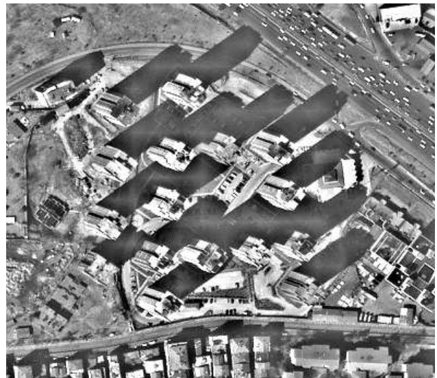
Figure 4. Extract of Wallis-filtered 11-bit Ikonos image. The radiometric filter enhances the existing texture patterns locally, leading to optimization of the contrast in the shadow areas.
