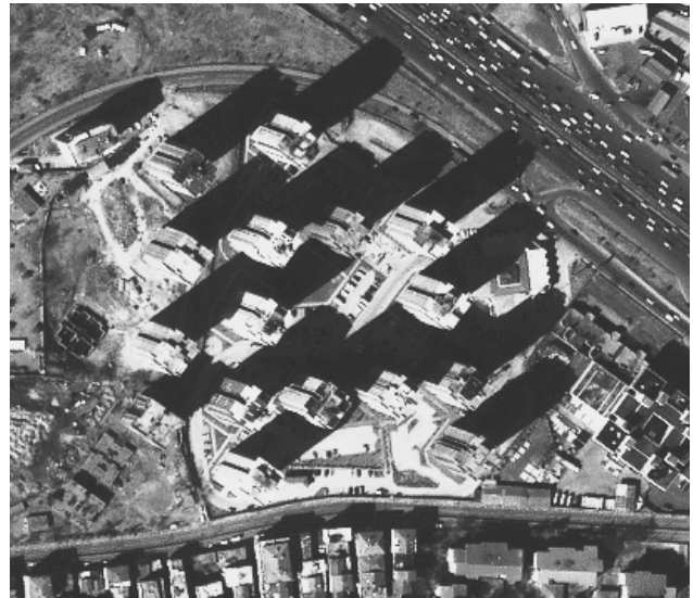
Figure 3. Extract of original 11-bit Ikonos image, illustrating an area with high buildings. There is very little contrast within the shadow areas, leading to mismatches during the image matching process.
