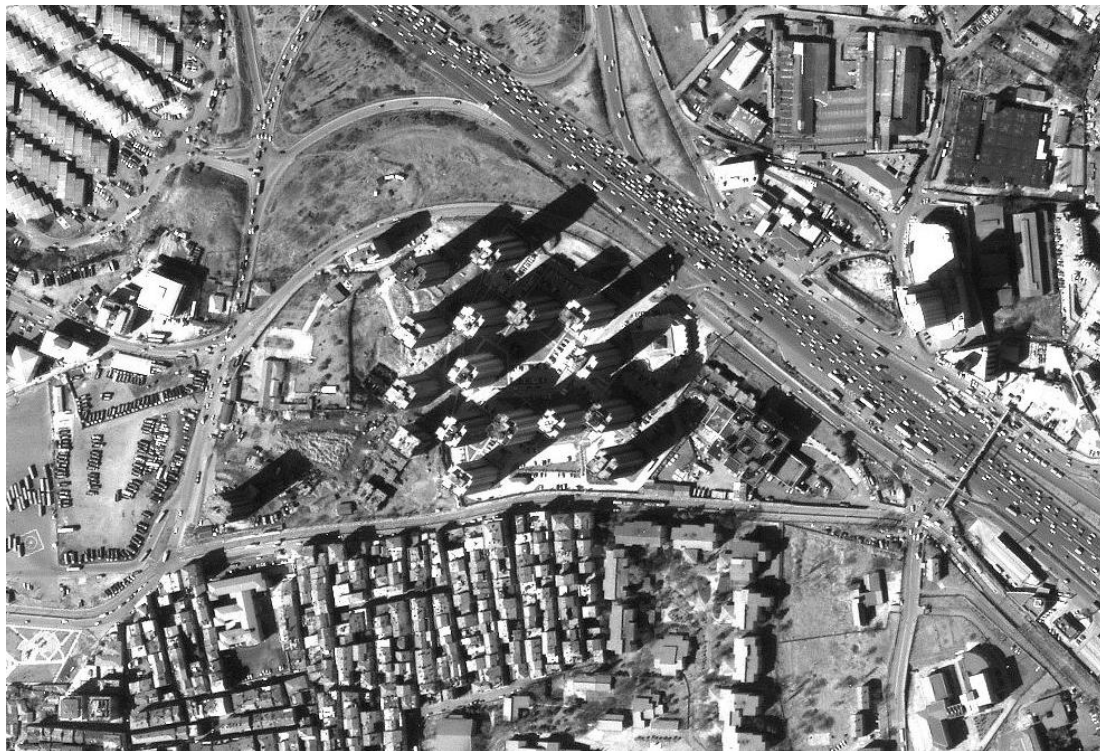
Figure 2: subimage of ikonos A: high buildings leading to huge image displacement, long shadows and occluded areas.
