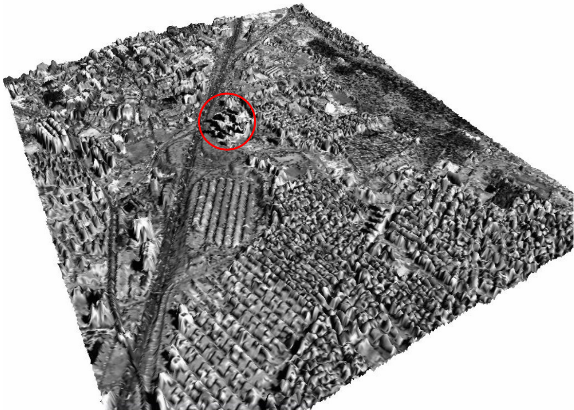
Figure 3: Part of drape (DSM overlaid with ortho image) created out of stereo couple AB. Due to big image displacement of the buildings shown in figure 2, mismatches lead to errors in the DSM.
